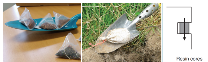
Fig 3. Tetrahedron-shaped synthetic tea bags used for Tea Bag Index (TBI) experiments; Resin bags for nitrogen leaching risk measurement; Installation of resin bags.
