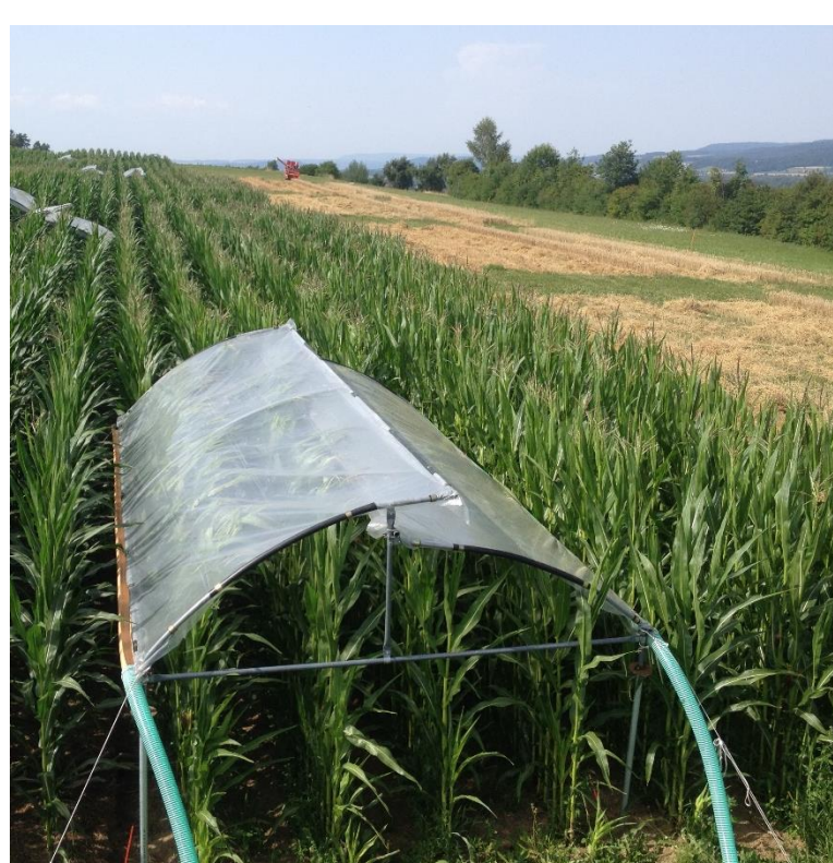
Fig. 2. Rain shelter used to promote drought at the specific farming system plots in field. Note the green tubes, their function is to capture the rain water and disposing it away from the plot, avoiding that it flows back and hinders drought.
