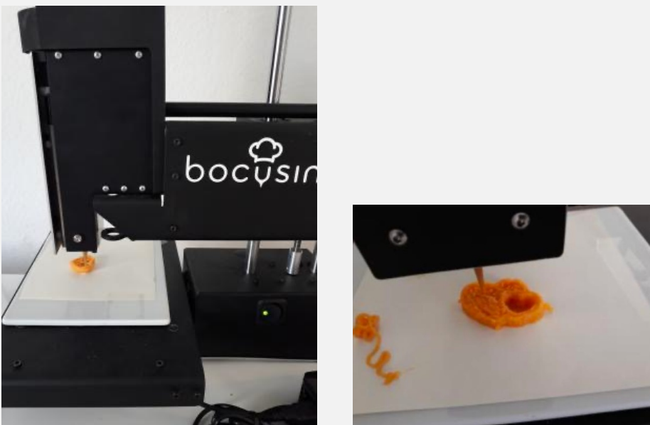
Fig 1. 3D printer shown to the participants, currently printing carrot puree in a heart shape. Used by the Texas Tech University to print the food presented in the survey. Credit: Paul Egan, Texas Tech University.
