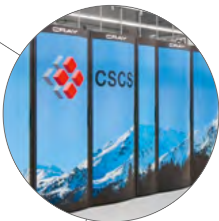
"Piz Daint", the high-performance supercomputer at the CSCS, processes vast amounts of data and enables simulations to be performed at an unprecedented degree of precision.
