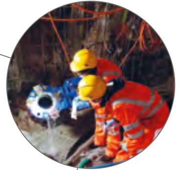
Sampling a deep borehole in the Bedretto Underground Laboratory for Geosciences and Geoenergies
