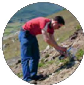
The lead content of a soil sample is determined using a mobile x-ray fluorescence device.
