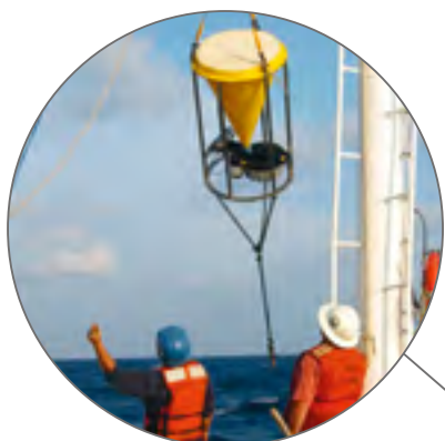
Lifting the sediment trap.
