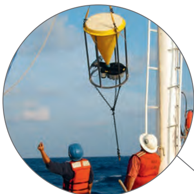
Lifting the sediment trap.
