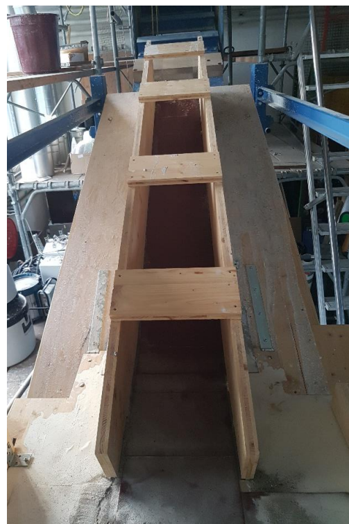
Figure 2. Channel of the debris flow flume with bottom covered in sandpaper to increase the basal friction.
