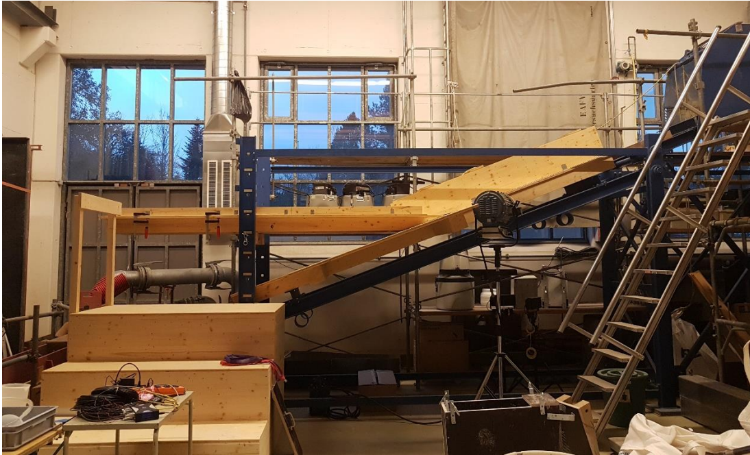
Figure 3. Side view of the WSL debris flow flume channel and deposition platform.
