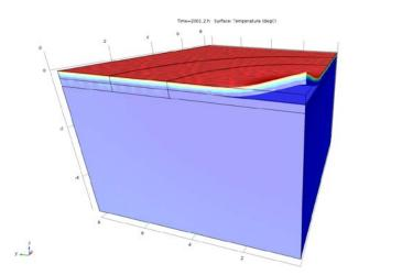
3D model developed in COMSOL Multiphysics correlates hourly bedrock temperature fluctuations with the buckling of a 0.5 m thick bedrock slab.
