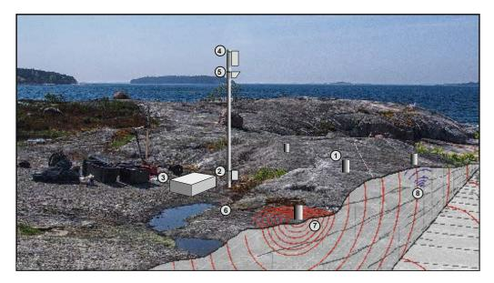
Schematic of the fracture monitoring installation
