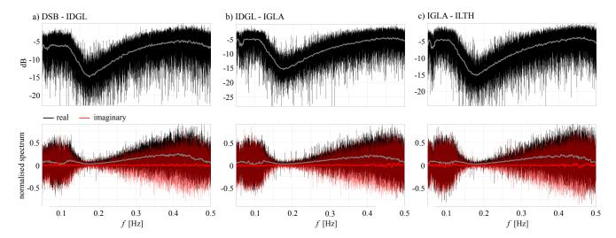
Figure 5. Frequency-domain propagation correctors  $g_{ik}$  for selected receiver pairs (i, k). Normalised amplitude spectra are shown above, and the separate real and imaginary parts below. As in the previous figures, smoothed versions of the spectra are shown for better visibility. Propagation correctors for other receiver pairs are very similar in character.
