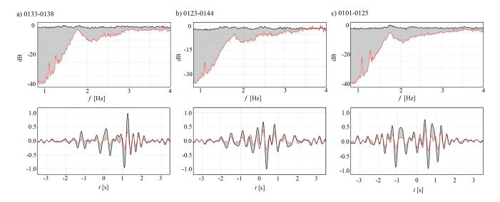
Figure 8. Amplitude spectra (top) and time domain waveforms (bottom) for noise correlations of Lost Hills station pairs 0133-0138, 0123-0144, and 0101-0125. Regular processing is shown in black, optimal processing in red. The difference between the two, shown in grey shading, estimates the unphysical component introduced by nonlinear processing.
