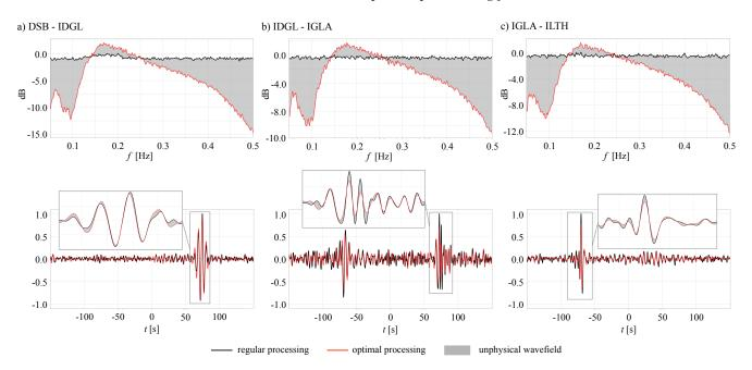
Figure 6. Amplitude spectra (top) and time-domain traces (below) of correlations for the same station pairs as in Fig. 5. Regular processing is shown in black, and optimal processing in red. The estimated unphysical wavefield, shaded in grey, is the difference between the two.
