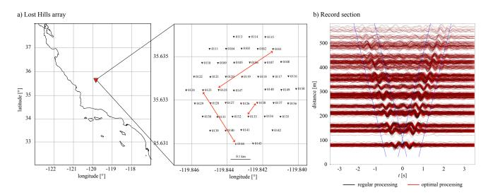
Figure 7. The Lost Hills seismic node array (Clayton, 2015). a) Geometry of the array, located north-west of Bakersfield in southern California. b) Record section showing regularly processed correlations in black (spectral whitening and rms clipping), and optimally processed correlations in red. For better visibility, traces are normalised to have equal maximum amplitudes. Examples of unnormalised traces are shown in Fig. 8 below for the station pairs indicated by red arrows in panel (a).
