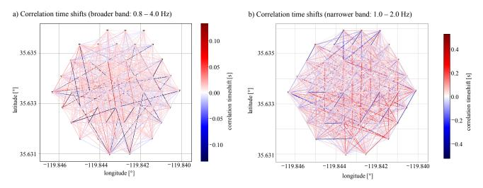
Figure 9. Unphysical surface wave traveltime biases introduced by nonlinear processing in a broader frequency band of 0.8 - 4.0 Hz (left) and a narrower frequency band of 1.0 - 2.0 Hz.
