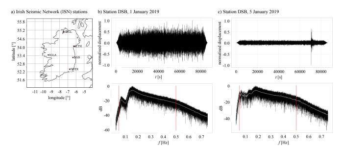
**Figure 3.** One-day-long vertical-component recordings on January 1 and 5, 2019, at station DSB, which is part of the Irish Seismic Network, shown in panel (a). Time-domain plots (top) display normalised displacement, and the frequency-domain plots (bottom) show normalised spectral amplitude. The grey line is a smoothed version of the spectrum, included for better visibility. The red vertical lines mark the boundaries of the frequency spectrum, used in the analyses below.
