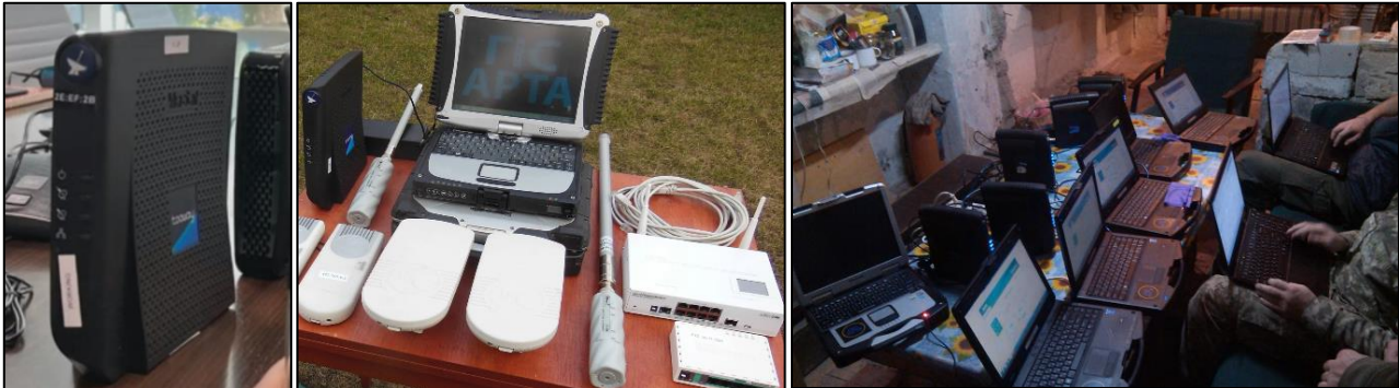
Figure 46-48: (left) Bricked ViaSat Tooway modem; (center) GIS Arta's satellite suite; (right) GIS Arta & ViaSat modem use in Ukraine
