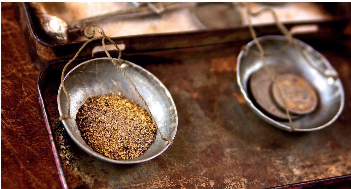
Local traders use a handheld scale or “flail scale” with coins and matches as counterweights to determine the weight of the gold. Photo: Enough Project
