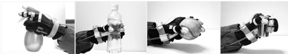
Fig. 1. Various grasping motions with Exo-Glove performed by subject with paralysis in the hand.
