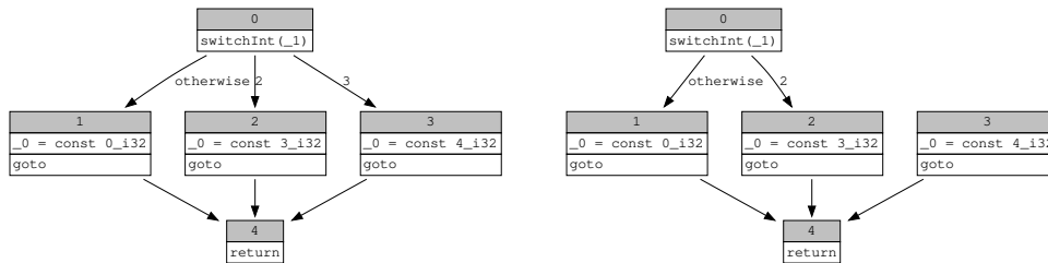
Figure 4.9: MIR of Listing 4.8 before and after optimization.
