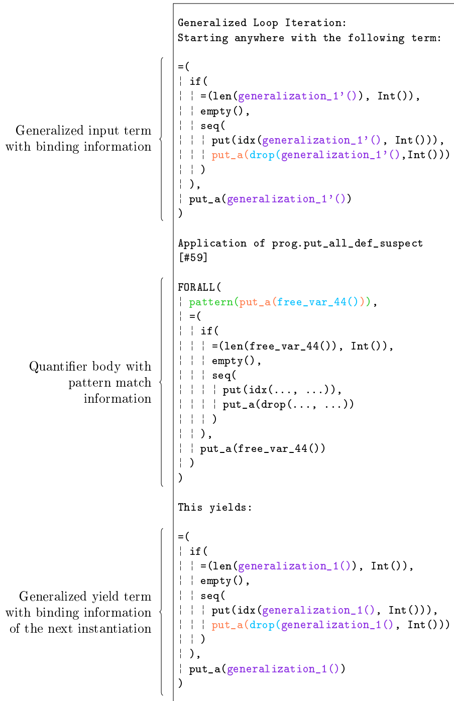
Figure 14: Generalized loop description of a loop of size 1. Note that the generalized input and yield terms do have the same term structure, but they differ in the concrete loop since the generalizations are from different iterations. This is a necessary requirement for a loop of size one, otherwise the instantiations would either not be looping or the loop would be longer.
