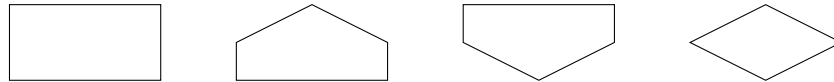
Figure 3.20: The shapes from left to right are used if all parents and children are displayed, some parents are not displayed, some children are not displayed, and some parents and some children are not displayed.
