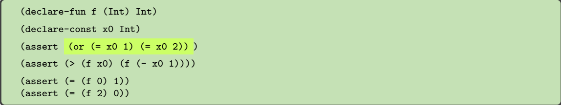
Figure 28: First (erroneous) approach for constructing a potential EXAMPLE for the input in Figure 27, where the term (x_0 = 1) \vee (x_0 = 2) provides a selection of values for the free variable x_0 . The EXAMPLE is satisfiable, because x_0 = 1 satisfies all the assertions.
