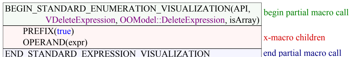
Figure 4.5: X-Macro example from Envision’s C++ code base showing the relationship between partial macros and X-Macro children .
