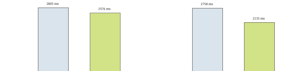
Figure 4.1: In order to analyze the impact of the newly added triggers, we verified sample programs with Boogie and Simplify and measured the time it took the process to complete. We have performed fifty test runs per program and then evaluated the average over all test runs. The first diagram depicts a small program with a couple of object instantiations and method calls, where a slight improvement of 8% could be determined (blue: average runtime without triggers, green: average runtime with triggers). The second diagram shows the results of a basic QuickSort algorithm, where field and array operations are involved. We could measure an impressive speed-up of 23%. The improvement might even increase if more axioms (in terms of number and complexity) are involved in the verification process. However, we did not perform any further in-depth tests to fortify these assumption.
