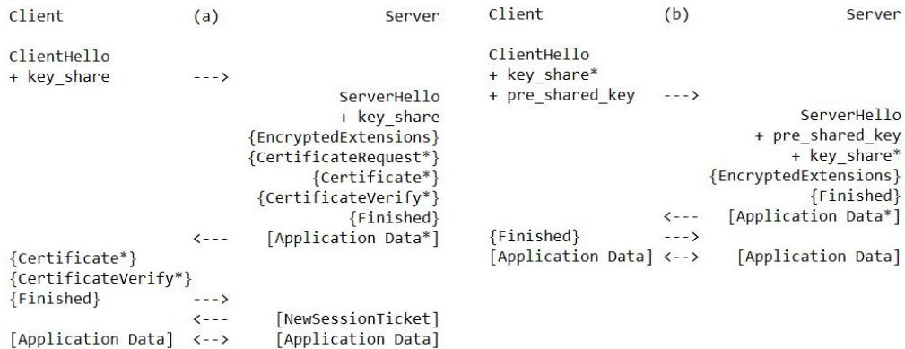
Figure 3.2: Handshake with PSK (a) Initial Handshake (b) Subsequent Handshake
