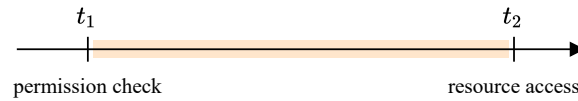
Figure 2.2: If the object reference can be changed between t_1 and t_2 , the permission check at t_1 can be tricked in regard to the access at t_2 .
