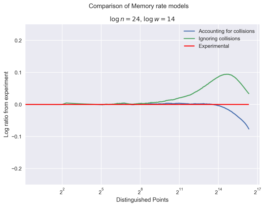
Figure 4.4: Ratio of prediction of Model 4.12 and Model 4.4 to actual fill rate. 'Ignoring collision' refers to Model 4.12 and 'Accounting for collisions' to Model 4.13. Actual is averaged over 100 runs. x -axis cut off at n\theta^2 . Log-Log scale.
