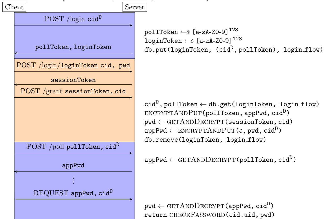
Figure 4.5: Desktop client login. The blue sections show the messages exchanged between the desktop client and the server. The orange section shows the messages exchanged between the browser and the server. The web client is identified by the identifier cid , and the desktop client is identified by the identifier cid D
