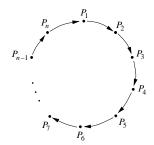
To distinguish the processes, each process has a unique identifier id with  $1 \le id \le n$ . The aim is to elect the process with the highest identifier as the leader within the ring. Therefore, each process executes the following algorithm:
