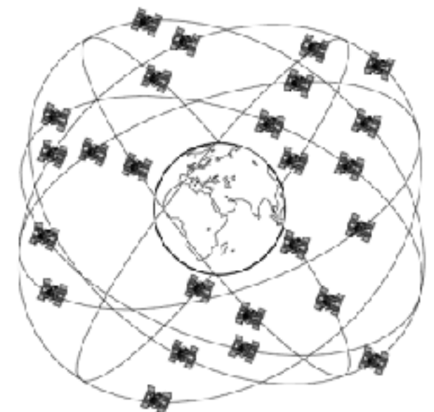
Figure 35: GPS satellites orbit the Earth on 6 orbital planes
