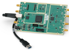
Figure 7.2: USRP software-defined radio with USB interface
