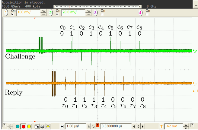
Figure 9: Oscilloscope trace of example messages exchanged in the implementation, and the values of the data symbols.
