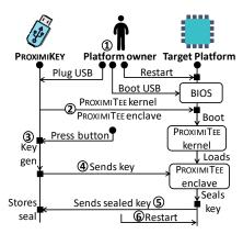
Figure 10: Boot-time initialization. The ProximiKey uses a minimal kernel Linux image to boot and load ProximiTEE enclave on the target platform and seal a platform specific secret to the ProximiKey memory.
