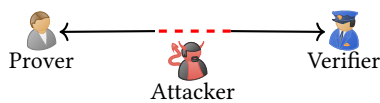
Figure 3: Mafia Fraud attack scenario against distance bounding and ranging. The attacker tries to reduce the time-of-flight measurement acquired by the verifier.
