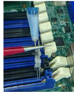
(a) A custom shunt probe. (b) Tweezers short-circuiting DQ_0 and V_{SS} .
