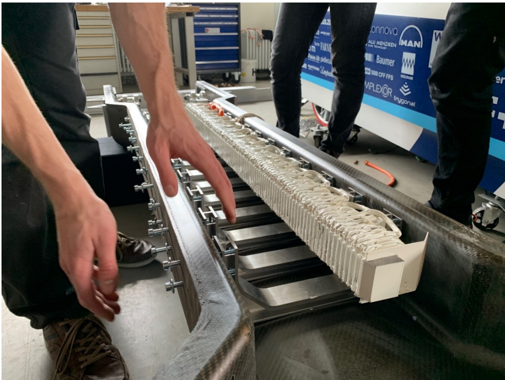
Figure 4. The core of the LIM2 (top) and one side of the LIM2 with the windings (bottom) is presented. More details can be found in the text.
