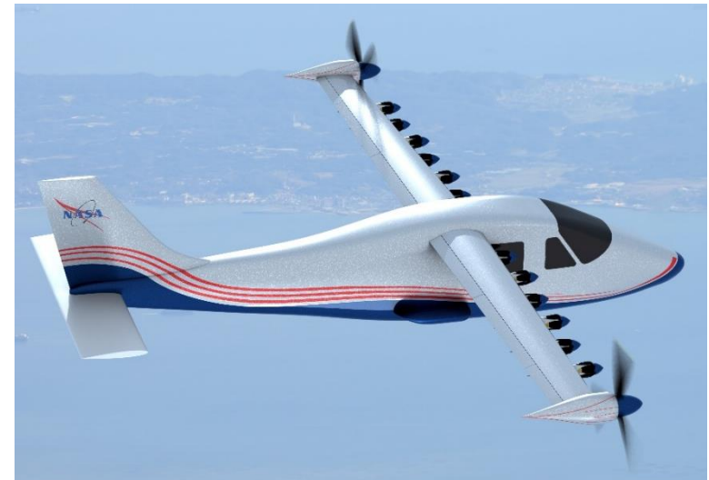
NASA's X-57 "Maxwell" will be a fully battery powered research aircraft using distributed propulsion.
