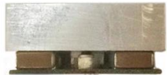
Side view of the switching cell with heat sink mounted to the SMT nuts with plastic screws
