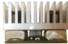
Front view of the heat sink with post contacting the GaN device (center)
