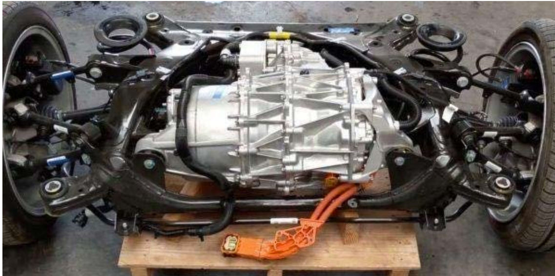
Tesla Model 3 Electric Power Train with SiC Inverter
