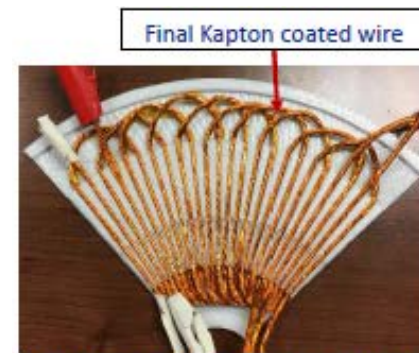
Quarter stator with cavities placing 0.06" Kapton coated Litz wire.
