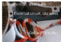
Direct Cooled windings
