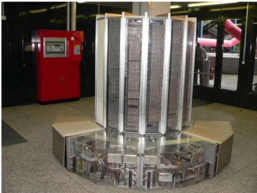
The Cray 1, a vector supercomputer. The first model ran at 80MHz but could retire 2 instructions/cycle for a peak of 160 MIPS. However, it could reach 250 MFLOPS using vectors.
