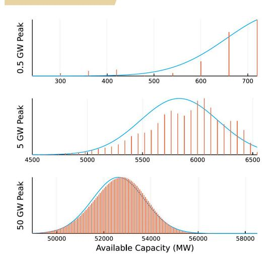
Distribution of total available generation capacity (rounded to the nearest full unit) for three system sizes
