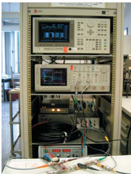
Labview-controlled Transmission Line Pulser developed in the thesis.
