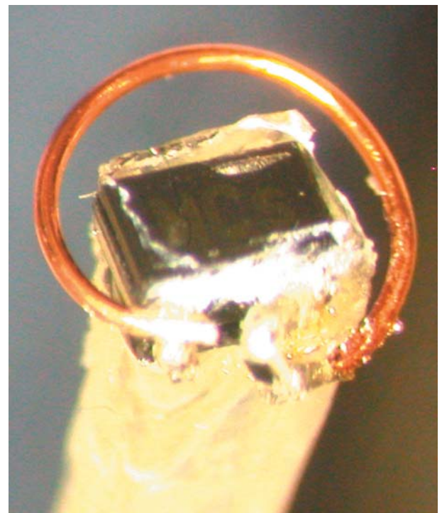
Sensor Head, loop diameter: 3.4 mm.
