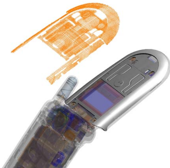
Schematic depiction of a shielding problem. Bottom: The upper shell of this flip phone is coated with a thin metallic shielding layer. Top: Voxel representation of the thin sheet.
