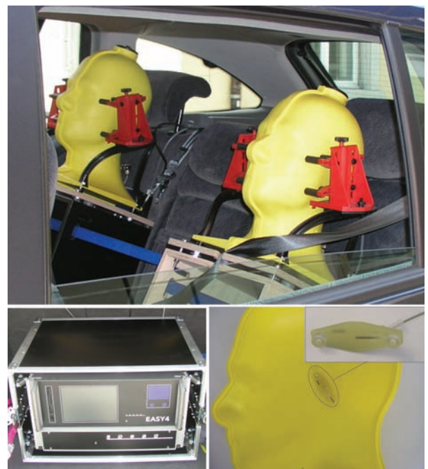
Top: Measurement system phantom heads mounted inside a car.
