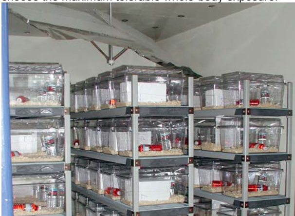
Reverberation chamber with cages containing phantoms.
