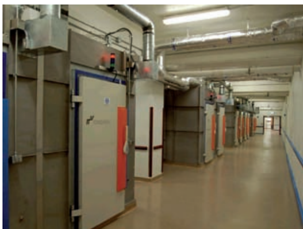
NIEHS, National toxicology program radio frequency exposure facility manufactured and installed by the IT'IS foundation.
