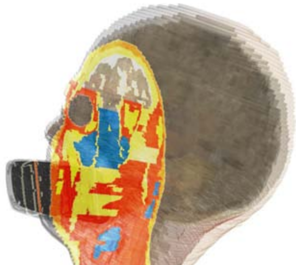
Human head and mobile phone. The FDTD grid contains about 700 million edges, but the update coefficient calculation completes in less than 1 minute. The highlighted cross-section shows part of the discretization.
