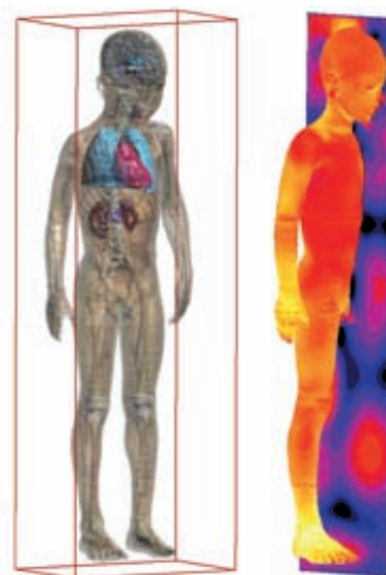
Left: Virtual Family Thelionius model inside a wave source box. Right: Thelionius model surface SAR and incident E-field view from an isotropic field incidence.
