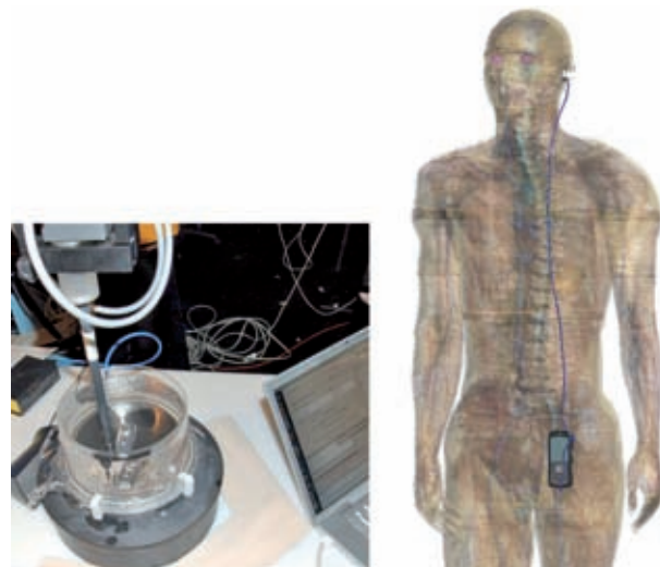
Left: SAR measurement of a wireless HFK in a novel vacuum phantom for devices partially surrounded by tissue. Right: Virtual Family Duke model with mobile phone and wired hands-free kit as used in the FDTD simulation in order to estimate human exposure in anatomically correct models.
