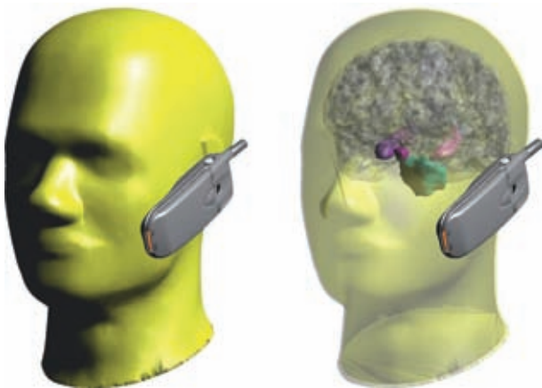
Left: Numerical model of the homogeneous SAM phantom head with a mobile phone attached. Right: Same SAM phantom with virtual head tissues and regions implemented using morphing techniques.
