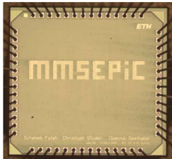
Chip photo of the SISO MMSE PIC detector. The 90nm CMOS ASIC performs SISO detection for iterative MIMO systems. The die size is 1.9 mm by 1.9 mm, from which only 1.5mm 2 are used by the detector.
