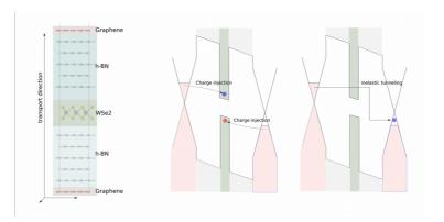
Left: an artistic rendering image of a photo-diode based on MoSe<sub>2</sub>/WSe<sub>2</sub> heterostructures. Center: a van der Waals structure composed of graphene/hBN/WSe<sub>2</sub>/hBN/graphene where transport happens vertically for electrical pumping. Right: band diagram of the van der Waals structure and two probable transport mechanism of the charged carriers.
