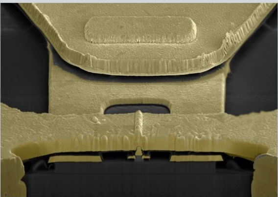
Cut away of a heterostructure bipolar transistor working at 700GHz
