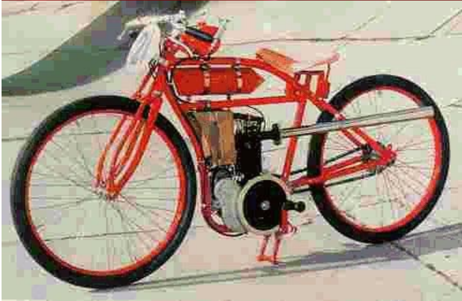
Racing bike; Opel 1922 Total weight 69 kg. Piston and crankcase made of Mg.
