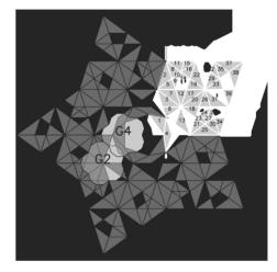
40Å x 40Å projection of a high-resolution electron density map with overlying pentagonal Penrose tiling (Niizeki modification).
