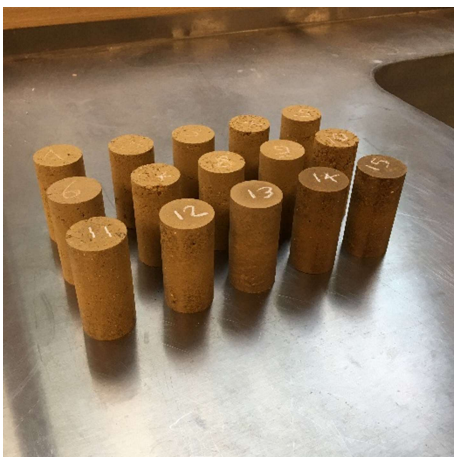
Figure 2 - (Left) Rammed earth cylindrical specimens. (Right) Specimen in unconfined compression test with DIC setup.
