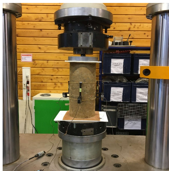
Figure 2 - Unconfined compression test on rammed earth cylindrical specimen equipped with extensometer sensors.
