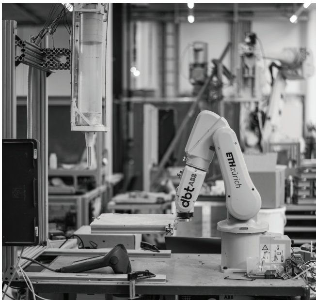
Robotic fabrication setup for the shading panel prototype.
