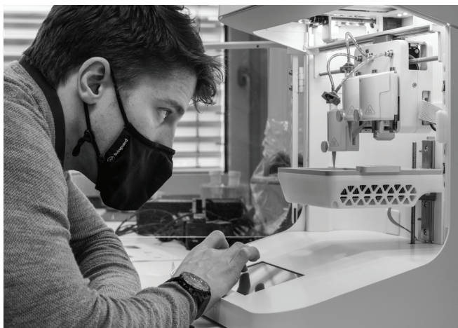
Elia Guzzi setting up the bioprinter with which they are processing their universal nanocarrier ink
