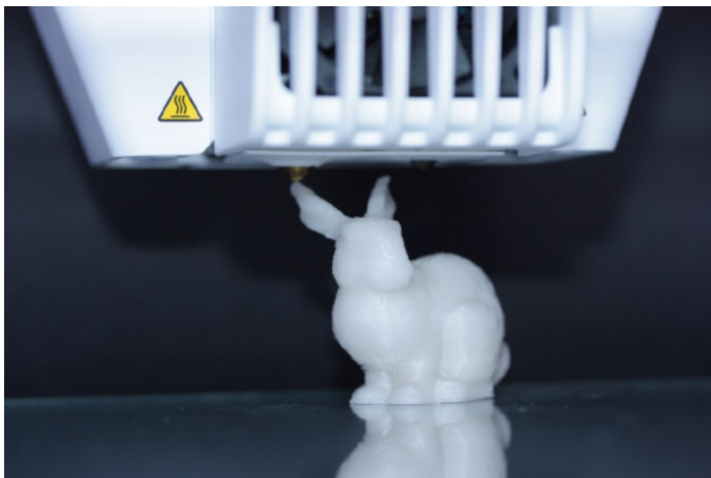
Fig.: Stanford Bunny printed with filament containing its .stl file in form of DNA.
