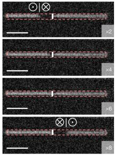
Magneto-optical micrographs demonstrating how a magnetic domain wall becomes inverted when pushed against a 50 nm-wide region engineered to have in-plane magnetic anisotropy (vertical white lines). The scale bar is 3  $\mu$ m. Reproduced from Z. Luo et al., Nature 579, 214 (2020).
