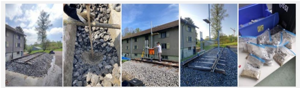
Test railway track: Data is gathered on a test railway track at the initial dry condition and, subsequently, at increasing water contents of the substructure over the steel, wooden, and concrete sleepers. The water content is assessed via ground truth tests in the laboratory on collected samples.
