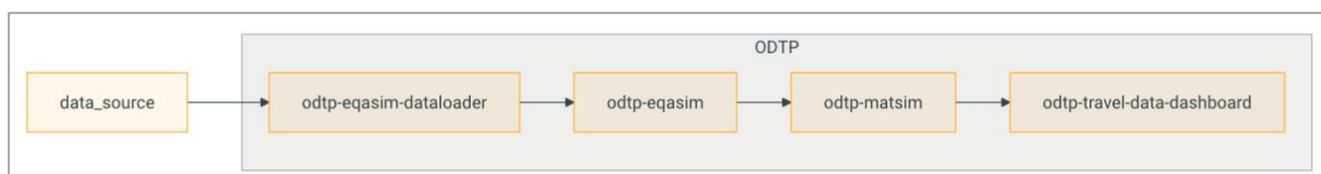
Figure 4. An example of an ODTP workflow to create and visualize a Digital Twin of the Swiss Mobility System.
