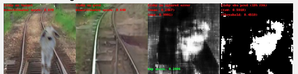
Fig. 4: Input image with an anomaly is reconstructed by the neural network. A difference measure highlights the anomaly as a white spot.
