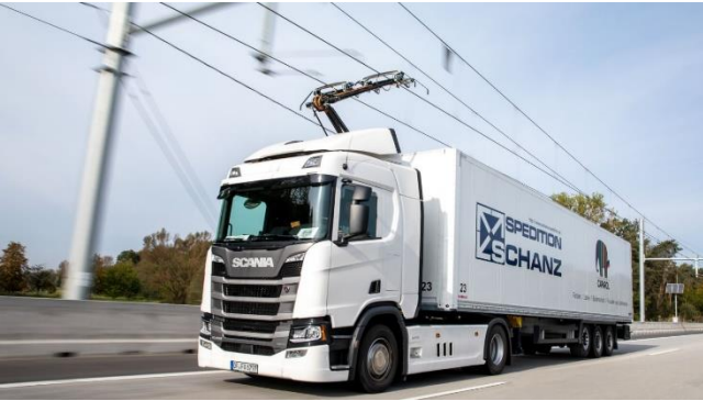
Overhead Catenary Electric
