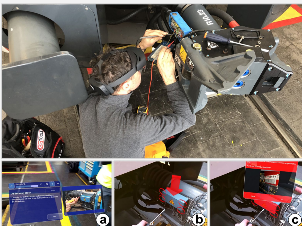
Fig 1: A technician performing a functional checkup of the train coupling while being guided with (a) augmented reality instructions. In the second study, the operator received (b-c) real-time feedback if a safety- or process-critical step was missed (e.g., switching off electrical fuses before working on electrical components).
